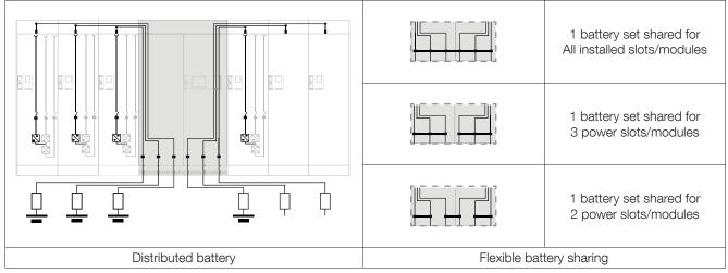
For full hot-scalability, the future battery protection should be prewired to the Power HUB, so that the battery set can be added later on.
