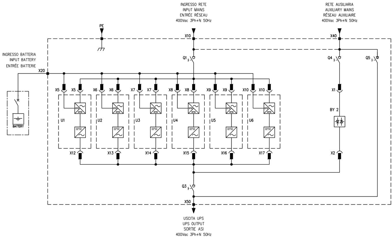
**System with 1+1 redundant bypass module**
