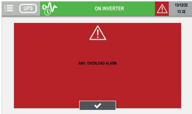
Tap on valid button to stop the buzzer and to close the popup message. The alarm page is automatically display after this action.
