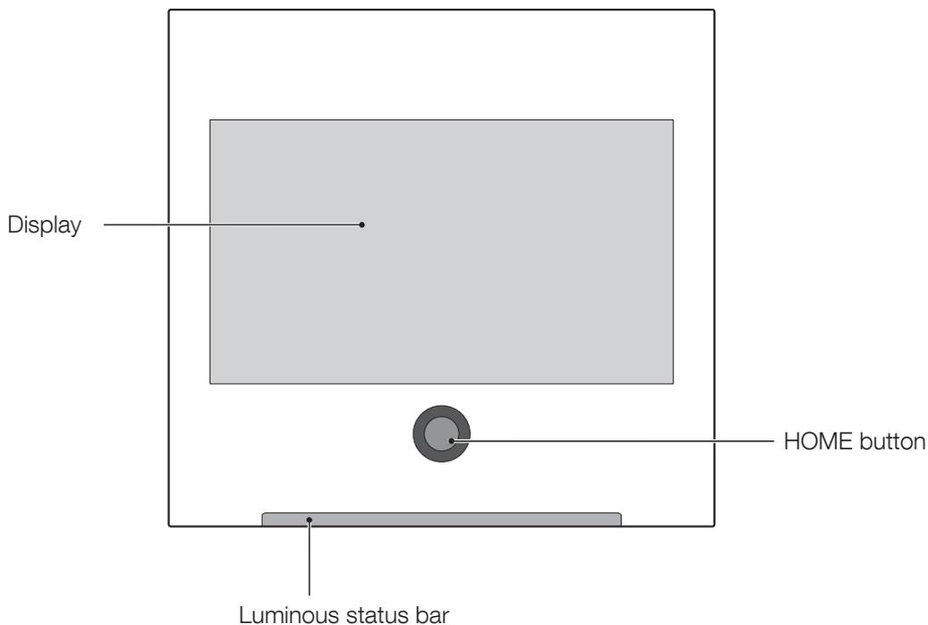
Only two elements are necessary to interact with the unit:
