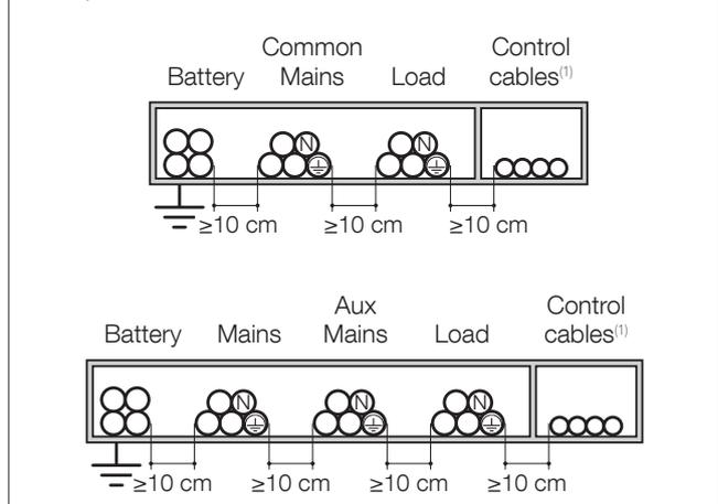
(1) Control cables: connections between the cabinets and each unit, alarm signals, remote mimic panel, connection to the BMS (Building Management System), emergency stop, connection to generator.
