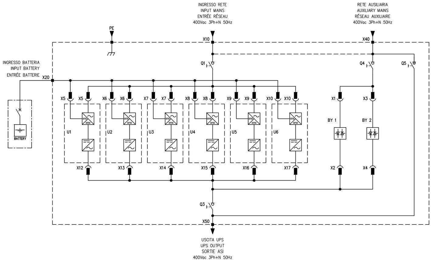
System with manual bypass, input, aux. mains and output switches and internal backfeed (with or without redundant bypass module).
