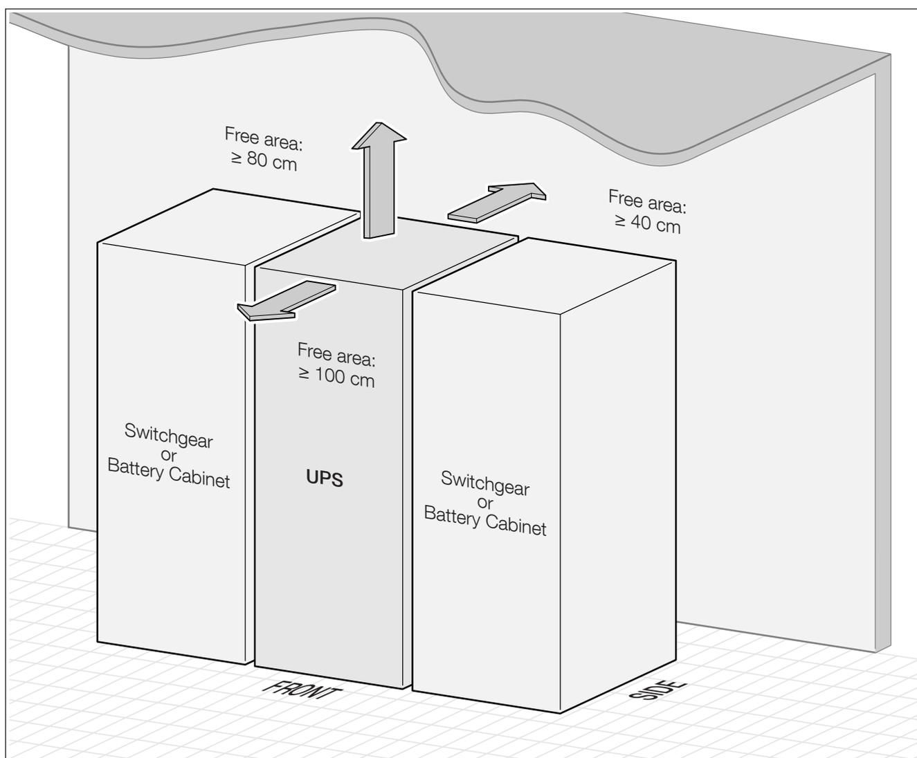
(1) Suggested Clearances in the worst case condition (@ Nominal Load and 40 C° ambient temperature). Contact SOCOMEC for different installation and application conditions.
