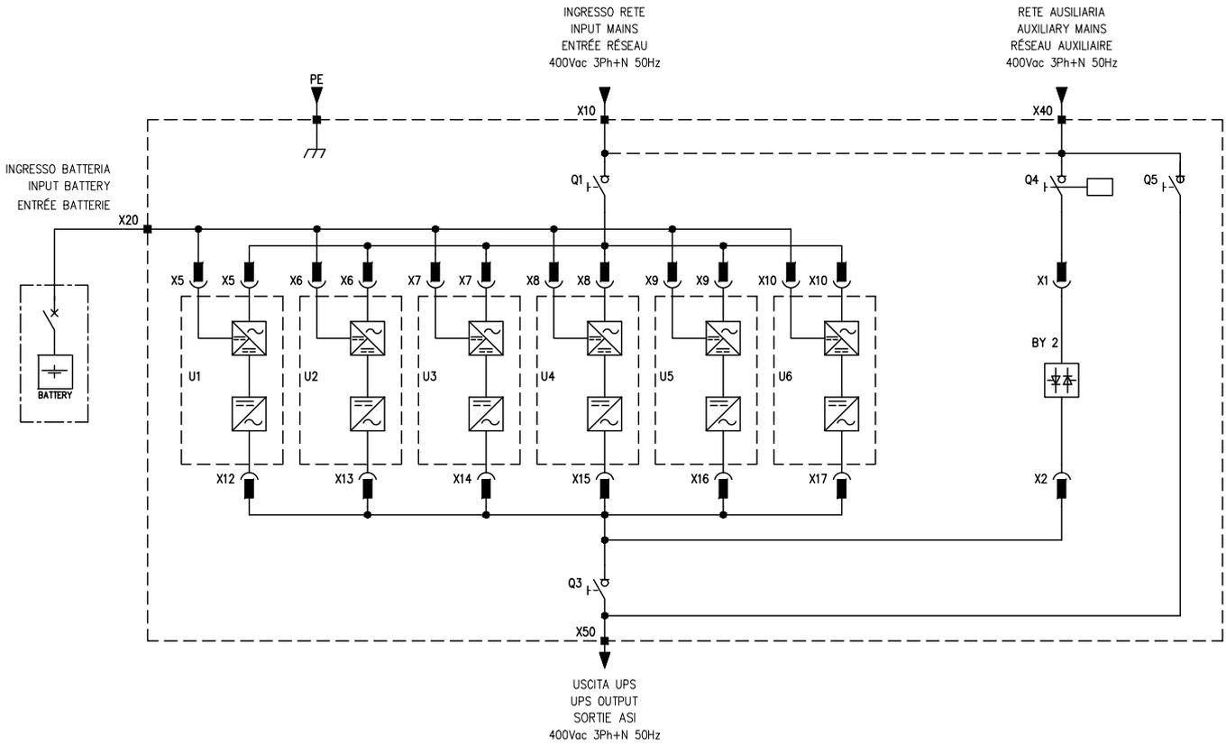
**System with internal backfeed and 1+1 redundant bypass module**
