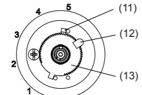
Figure 3: Adjusting wheels for temperature limitation (as-delivered state)
