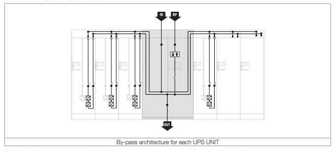
The above drawings show simplified diagrams for separated inputs (Rectifier / Bypass).
