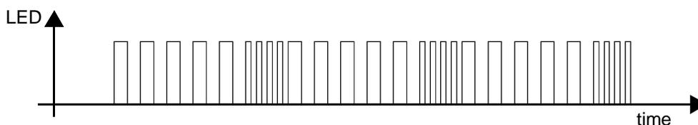
**Value transmitter: readjustment by long push-button press**
