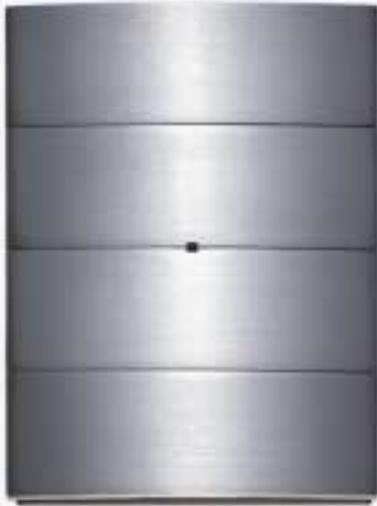
The B.IQ push-button comfort is plugged onto a flush-mounted bus coupling unit (flush-mounted BCU). The push-buttons of the device can be programmed for the following functions: switching, dimming, blind/shutter control, value transmitter, light-scene recall, forced guidance and control. Push-button assignment is free and fixed in the project.
