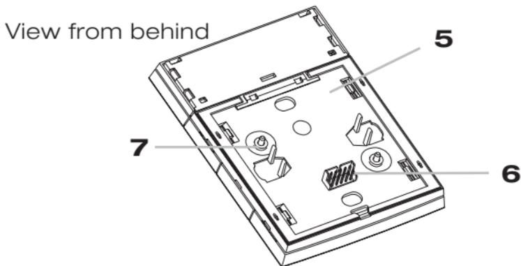
The 4/5gang push-buttons RTR are installed in the same way. A bus coupling unit flush-mounted plus is required.
