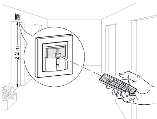
Figure 9: Using the hand-held transmitter
