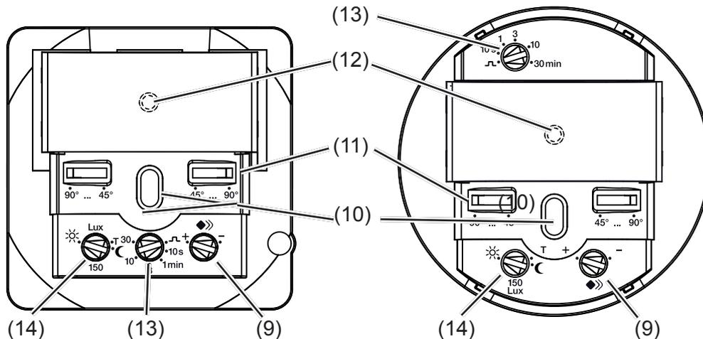
Fig. 5: Operating and adjustment elements of the bottom part of the application module
