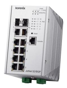
Korenix JetNet 5210GP, the DIN-Rail type industrial Gigabit Managed PoE Switch is designed with eight 10/100/1000TX ports, two Gigabit RJ-45 / SFP combo ports. JetNet 5210GP is the first industrial ethernet switch compliance with IEEE 802.3af/at/bt, each ethernet port can max supports 90W for PD, and total budget up to 480W 'Note.
