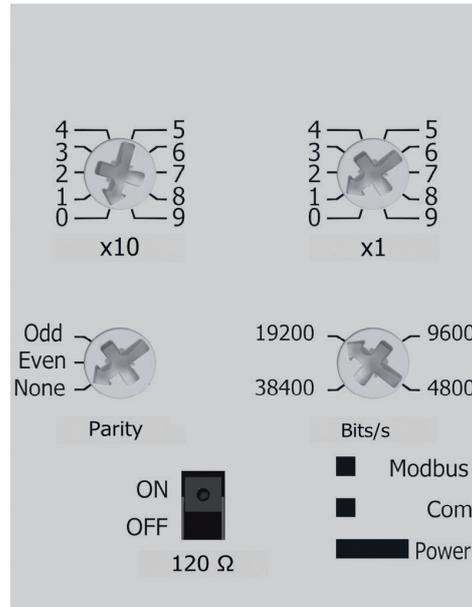
The parameters of the Modbus communication module can be adjusted on the front face using the adjustment dials and selector:
