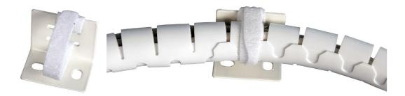
The ceiling fixing accessory can be used to mount a set of cables in a protective spiral wrap to the ceiling of a building. The fixing accessory can be attached to cable trays, lighting suspension rails, or other supportive structures. The spiral wrap can be secured to the fixing accessory with velcro.
