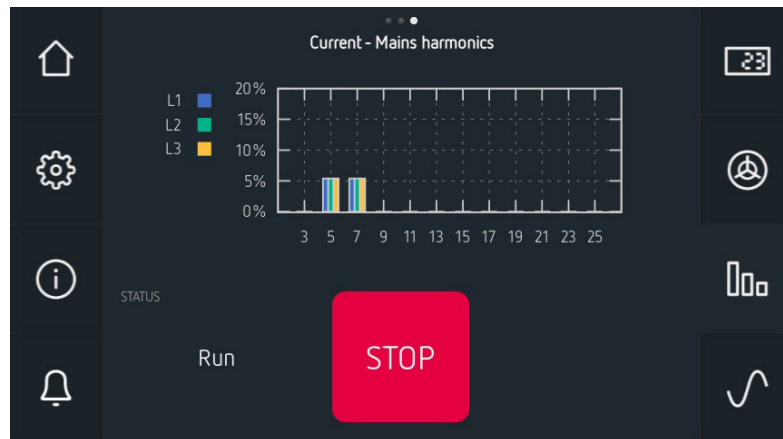
Figure 66: Display of the Mains harmonics.
