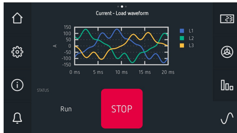
Figure 68: Wave shape of Load current.
