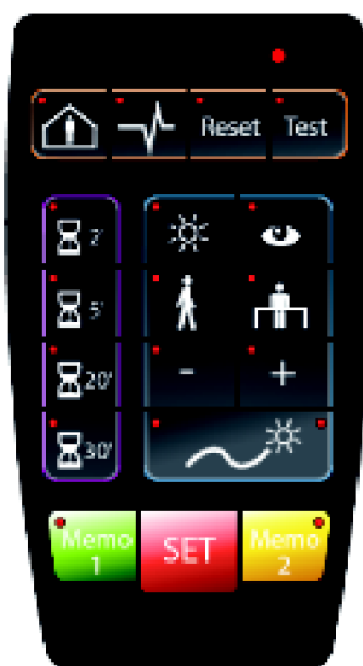
Installer remote control
