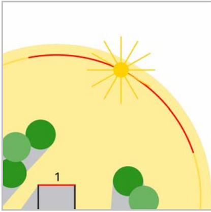
For facade 1, shading must only be active in the azimuth marked red, as the sun can then shine on to the building without obstruction
