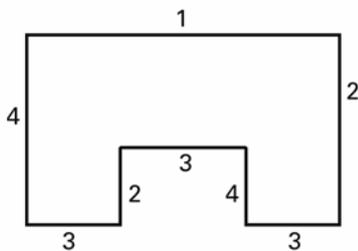
Even in buildings with a U-shaped layout, only 4 facades have to be controlled differently, as several have the same alignment.
