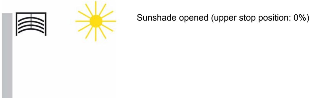
If the lower stop position is to be approached, this is specified to the blinds actuator as sun position "100%" or it will report reaching the lower stop position (i.e. sunshade fully closed) using this value. If blinds are moved down from the upper stop position, the slats first turn into an almost vertical position and the sunshade moves with closed slats to the lower stop position.
