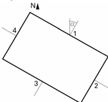
The facade orientation corresponds to the angle between the North-South axis and the facade vertical. The angle  $\alpha$  here is measured in a clockwise direction (North corresponds to  $0^\circ$ , East  $90^\circ$ , South  $180^\circ$  and West  $270^\circ$ ).
