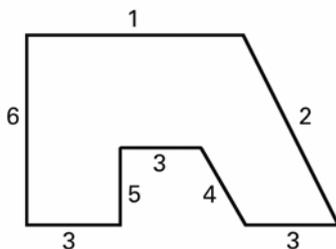
In buildings with an asymmetrical layout the facades with a non-right-angled orientation (2, 4) must be controlled separately.
