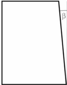
If a facade surface is not oriented horizontally, this must be taken into account. A forward inclination of the facade is counted as a positive angle; a backwards inclination (as in the picture) as a negative angle. This also allows a sunshade of a window built into a sloping roof surface to be controlled according to the current position of the sun.
