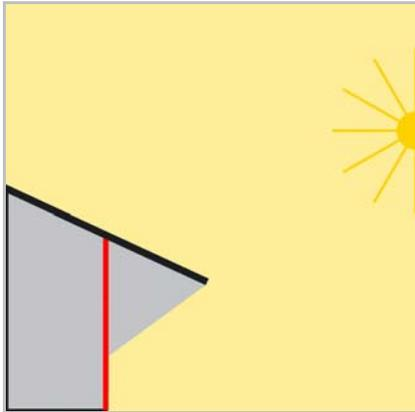
When the sun's position is high, the facade is only shaded by the roof overhang. Shading is only necessary if the sun is low (in the figure approx. below 53°).
