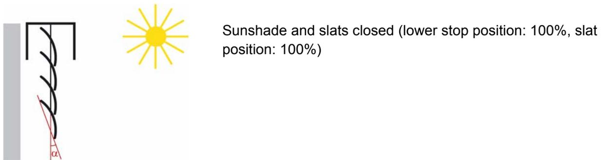
From its "vertical" position (completely closed, 100%) the slats can be adjusted to their horizontal position (fully opened, 0% or  $\alpha = 90^\circ$ ). For this, the drive used for the blinds defines whether this adjustment can take place almost continuously in many small steps (as with SMI drives, for example) or whether it is only possible in a few large steps (as with most standard drives).
