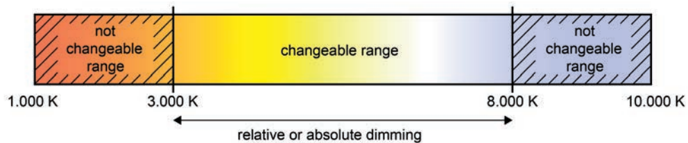
Figure 37: Automatic adjustment of the colour temperature to the set brightness Example in the maximum brightness and colour temperature range
