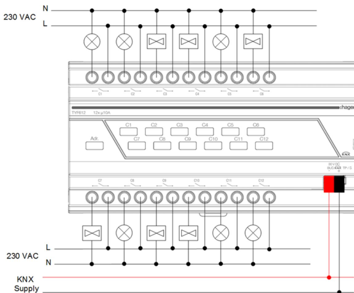
**Fig21. Connection Diagram Example Configuration 1**
