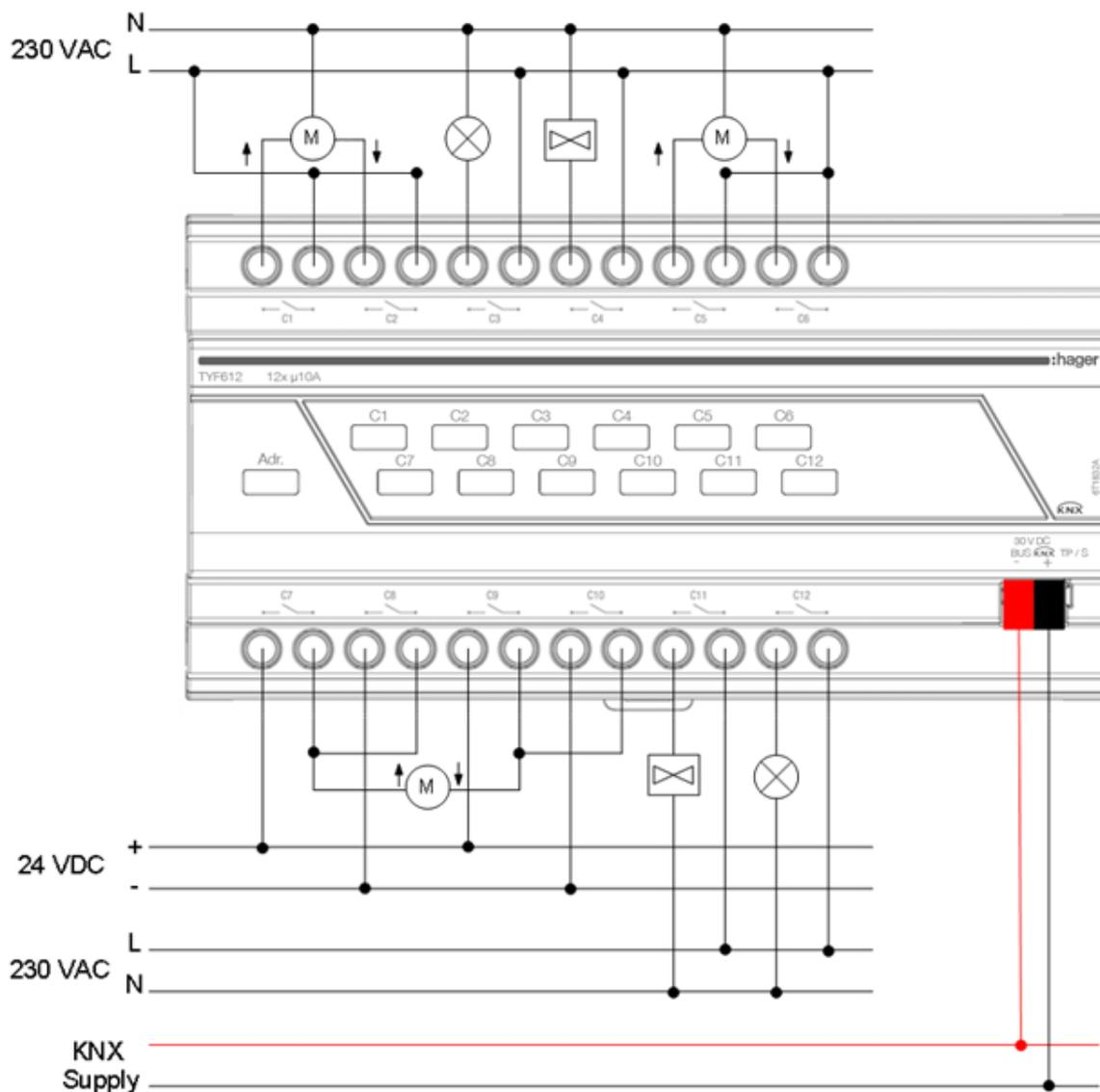
**Fig23. Connection Diagram Example Configuration 3**
