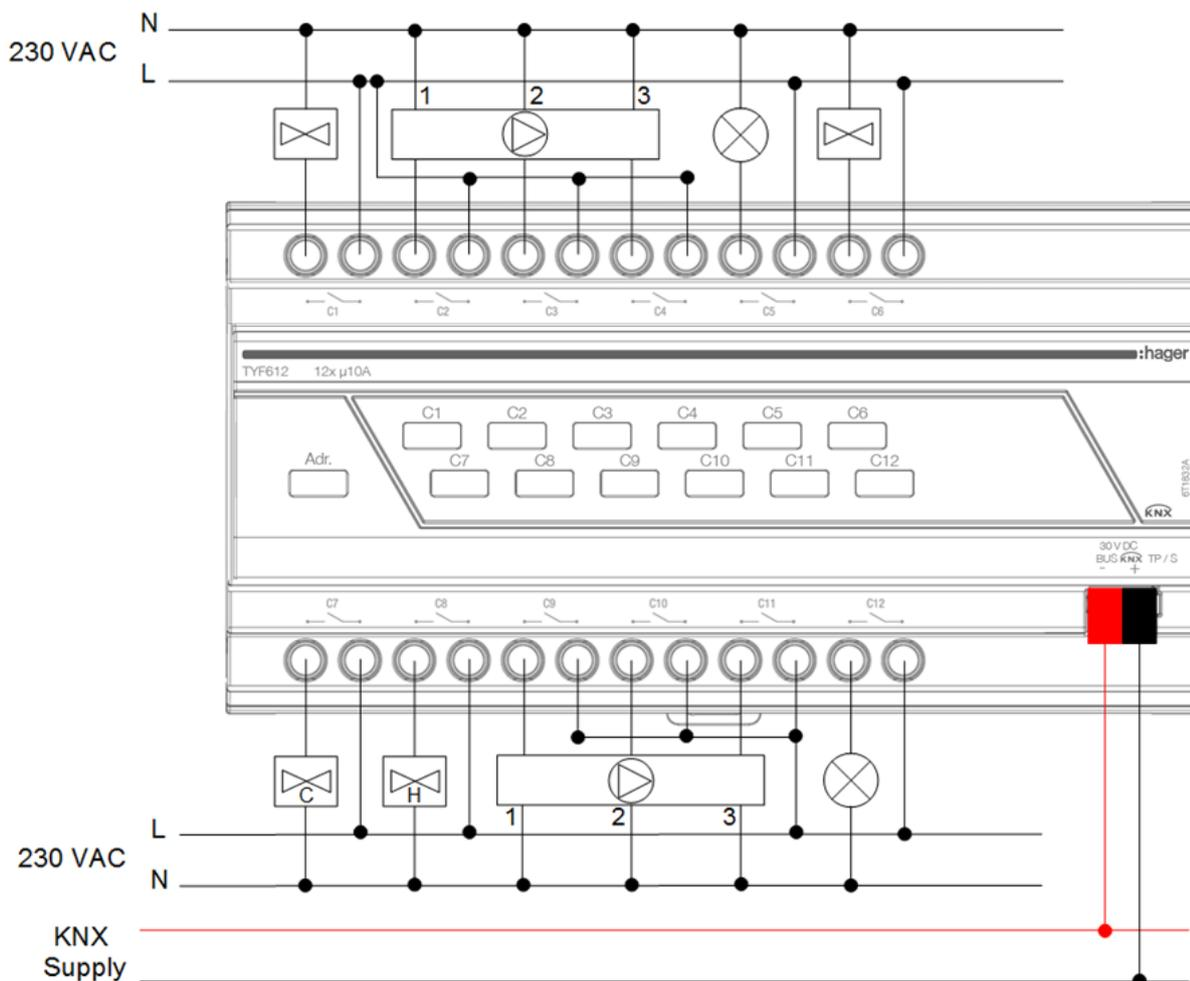
**Fig22. Connection diagram example Configuration 2**
