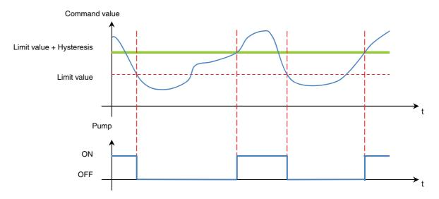
This object is used to send a pump control for the device on the KNX bus for the direct control of a heating or cooling circulation pump. The pump is activated by the product only if one of the configured values for the assigned outputs exceeds one of the defined limit values with the addition of the hysteresis. Pump deactivation occurs as soon as the value falls below the limit value.
