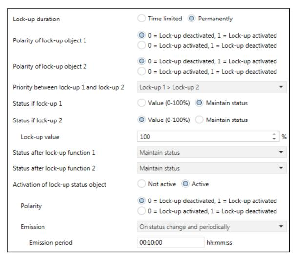
The Lock-up function is used to lock the output in a predefined state. The Lock-up prevents actuation until an unlock command has been received. The Lock-up duration can be set.
