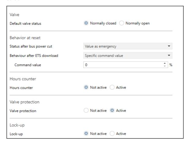
This parameter window is used to set the device outputs. These parameters are available individually for each output.
