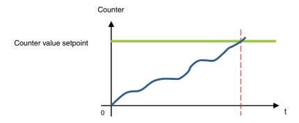
The counter starts to count up from the value 0. As soon as the counter setpoint (**Hours counter setpoint** object) is reached, the **Hours counter setpoint reached** object is set to 1 and sent to the bus.
