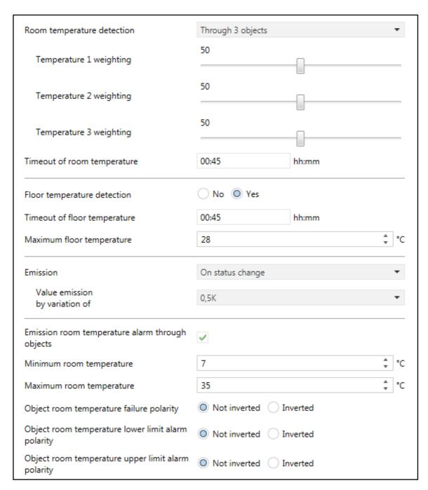
The thermostat detects the room temperature using up to a maximum of 3 external temperature sensors.
