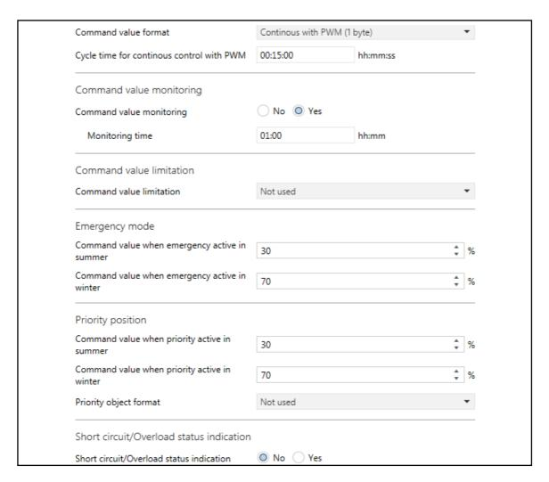
The product receives information from the KNX bus in 1 bit or 1 byte format from a KNX room thermostat for example. In general, based on room temperature, the regulator determines the values to be sent to the output product. The latter controls it valve outputs according to the data configured in ETS.
