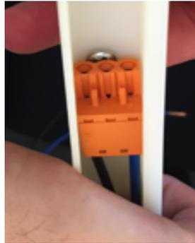
Integrated cable duct in the central area below the mounting rail
