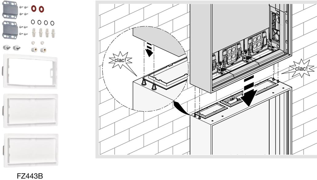
FWQ distribution boards can be mounted above each other with the FZ44xS accessories set. The third digit in the reference stands for the field width; **FZ443S** is suitable for connecting 3-field cabinets (800 mm width) above each other.
