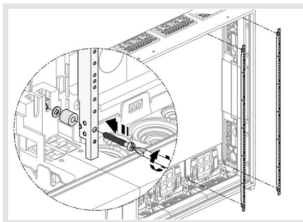
These panels can be easily fixed with the supplied 34.5 mm univers fixing screws and locknuts.
