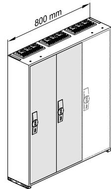
**Example:** To retrofit cabinet FWB53K5 (height 5 and width 3) with transparent doors, the door references FZ143N and FZ106N have to be ordered according to the table.
